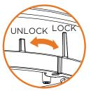
Adjust the camera modules' position and angle and complete the installation by placing the dome cover on the camera. Secure the dome cover to the camera base using the screws included with the camera. See the camera's QSG for more information.
