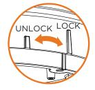
Adjust the camera module positions and angles, then complete the installation by placing the dome cover on the camera. Secure the dome cover to the camera base using the screws included with the camera. See the camera's QSG for more information.
