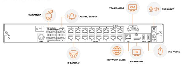
To prevent the NVR from overheating, do not operate it in an area that exceeds the maximum recommended ambient temperature of 104°F (40°C). To prevent airflow restriction, allow at least 3 inches (7.6 cm) of clearance around the ventilation openings.
