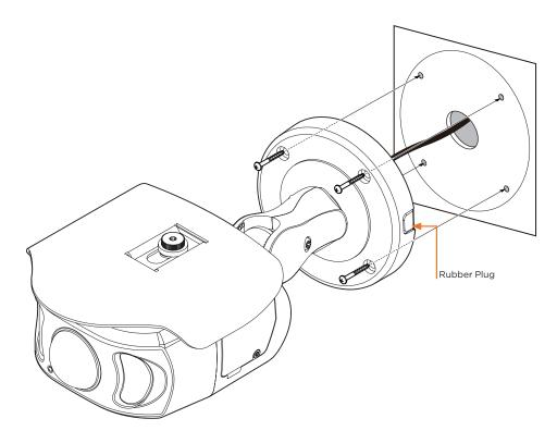
NOTE: Remove the rubber plug on the side of the camera's bracket and use the gap as a cable guide to prevent cables from getting caught between the camera and the mounting surface.
