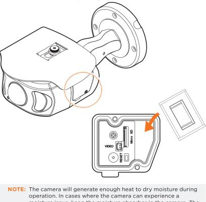
moisture issue, keep the moisture absorber in the camera. The moisture absorber has an approximately 6-month life cycle. WARNING: Install the moisture absorber when mounting the camera to prevent image performance issues and damage to the
